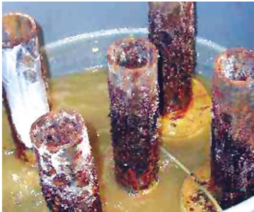
(Left) Insulated pipes in a 5% aerated salt bath. (Center) Same pipes 365 days into test. (Right) Pipe inspection after 365 days in salt solution. No corrosion in surface conversion treated areas.
