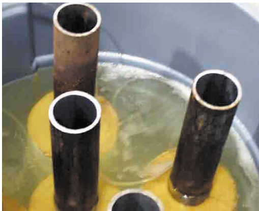
(Left) Insulated pipes in a 5% aerated salt bath. (Center) Same pipes 365 days into test. (Right) Pipe inspection after 365 days in salt solution. No corrosion in surface conversion treated areas.
